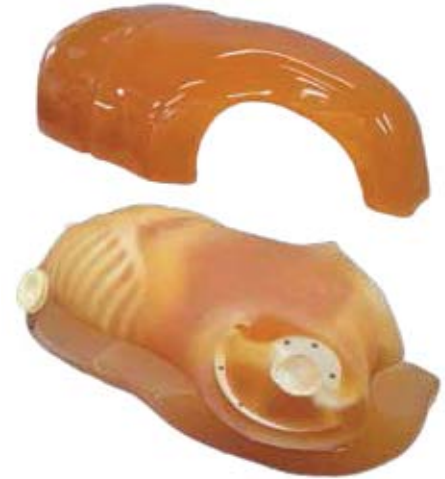
Body plates to simulate a body of BMI 30 The body plate provides the phantom with a variety of body shapes.
