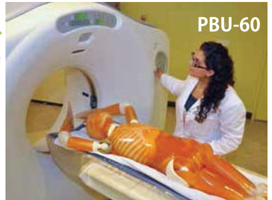
PBU-60 has full internal organs with proper HU numbers.
