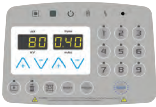
Operator Control Panel
